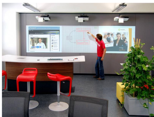
(a) The discussion room is equipped with a large interactive wall-mounted display. Users can interact with the content during meetings by using a digital stylus. In addition, the table enables meeting participants to connect their laptops and share content to the public display.
