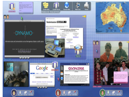
(b) Dynamo [Izadi et al., 2003] is a communal display designed for the purpose of exchanging digital media spontaneously. Users can select an area on the display as their private workspace, and can also provide access rights to others over their workspace and shared content.
