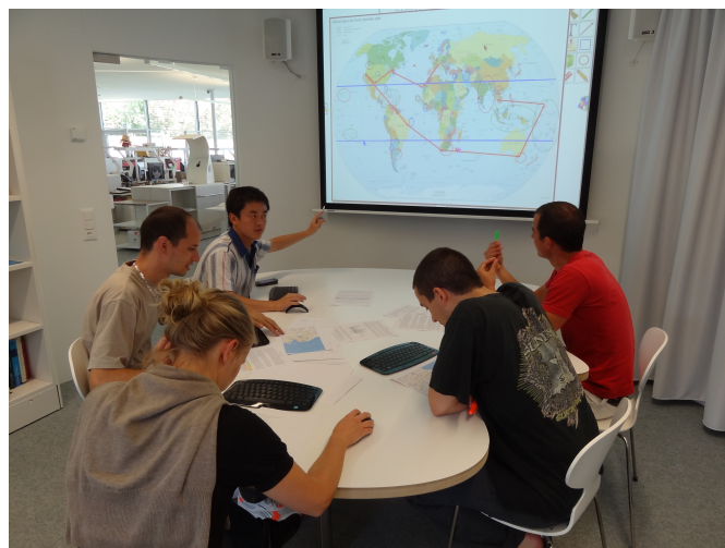
Figure 5.1 – The Mouse & Keyboard setup of MeetHub 1.0: Each group member was provided with a wireless mouse and a keyboard that were color coded. The users can interact with various tools and artifacts over the shared workspace (the vertical wall-mounted display) via their mouse pointer in the color of the device color code.
