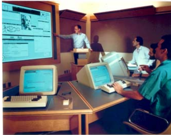
Figure 2.3 – The Colab Meeting Room [Stefik et al., 1987]: The meeting room at Xerox PARC designed for small collocated groups of 2 to 6 participants using a networked workstation. Besides individual workstations, the room is equipped with a large wall-mounted touch-sensitive display, and a stand-up keyboard.
