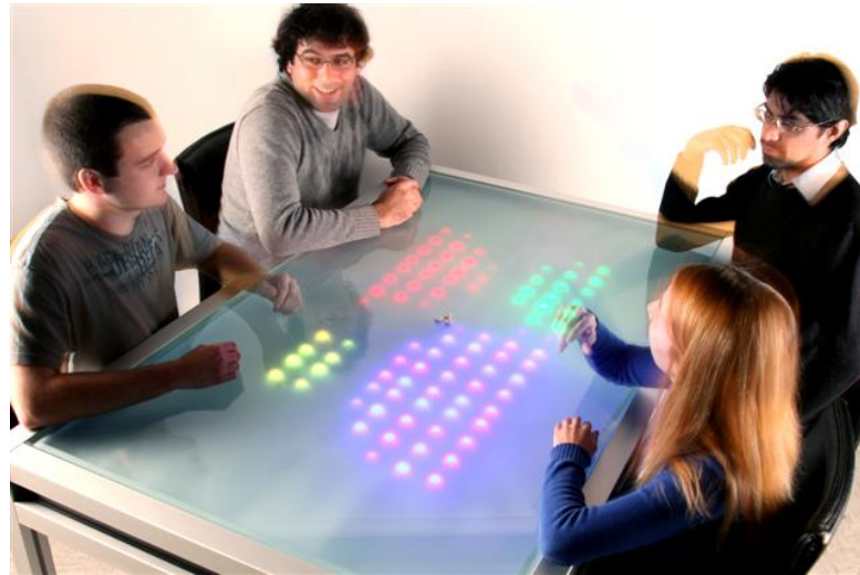
Figure 2.8 – Reflect Table [Bachour et al., 2010] is a group mirror, that visualizes the speech based participation information as territories of different color in front of the meeting participants in a semi-ambient way. The three microphone array situated at the center of the table in tandem with a selective filtering technique can accurately identify the direction of speech and the current speaker.
