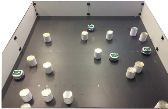
Figure 11.3: Arena with 15 obstacles and four Khepera III robots performing one of the obstacle avoidance algorithms learned.
