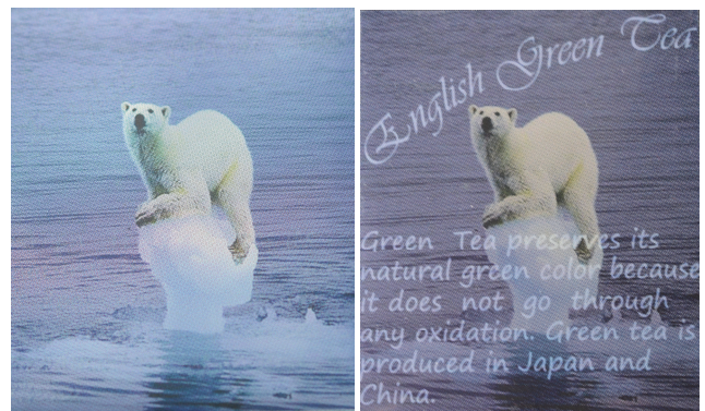
Figure 9: Photograph of a color print with the message “English Green Tea” hidden in specular viewing mode (left, exposure 1/400 s, aperture f/14) and revealed in non-specular viewing mode (right, exposure 1/50 s, aperture f/14). The mask values are set to 0.75 for the message text parts and to 0.32 for the background image. Therefore, in non-specular viewing mode, the text lightness is raised and the background image lightness is decreased. Original photograph by Arne Nævra, with permission.
