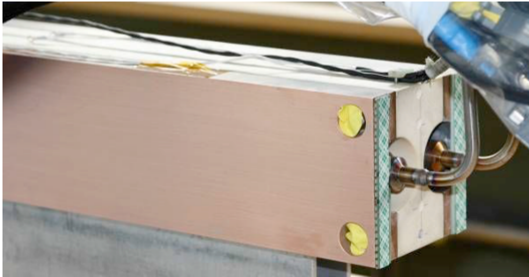
Figure 6a LTS sample upper terminations (facing the transformer) with helium pipes
