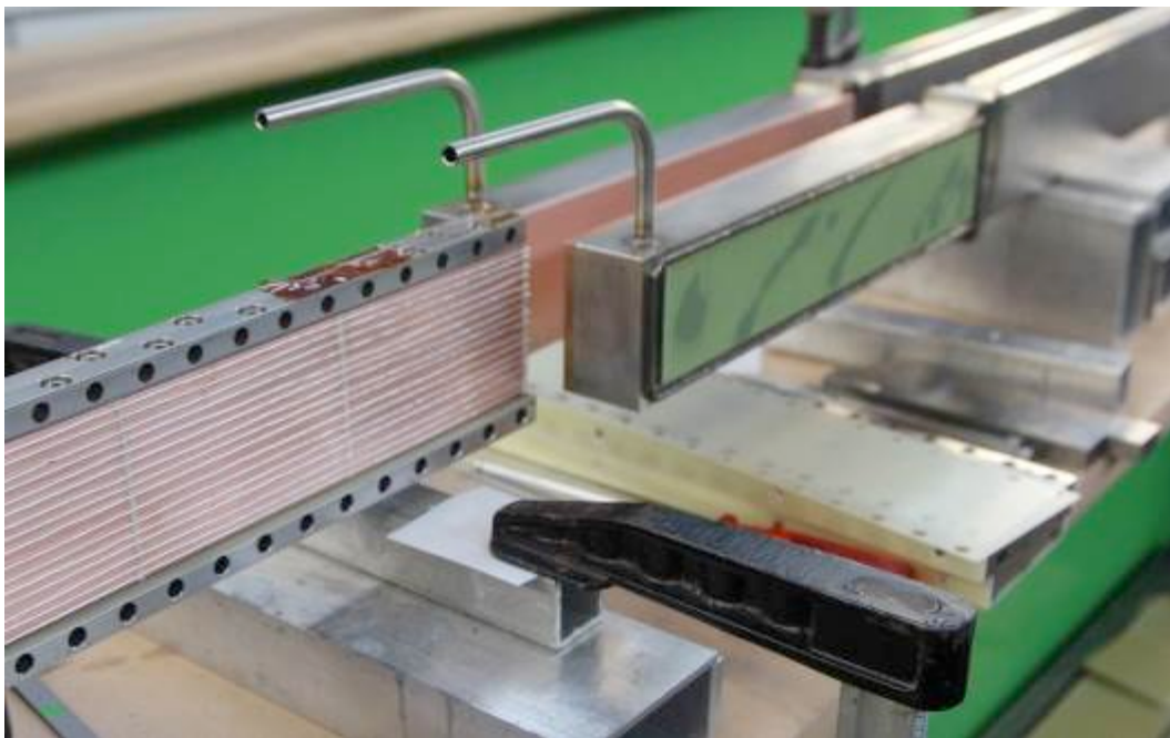
Figure 6b HTS sample upper terminations with piping and terminations of HTS adapter (left)
