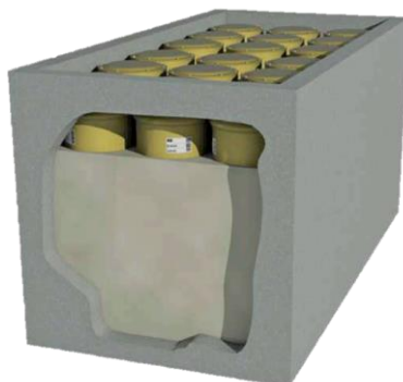
Figure 2.2 Drums containing solidified low- and intermediate-level will embedded by a mortar in a cement canister. These structure will be then place in deep geological repositories, after having backfilled galleries with a special type of mortar (Nagra, 2013).
