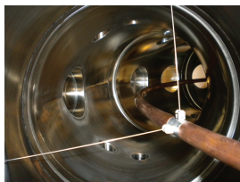
View of the copper wire inside the vacuum vessel of TORPEX.
