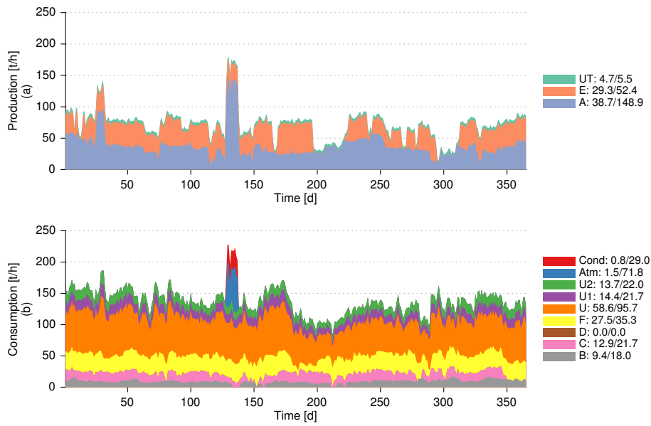
Figure 2.12 – Measured 5 barg steam consumption (a) and production (b) in Site P.
