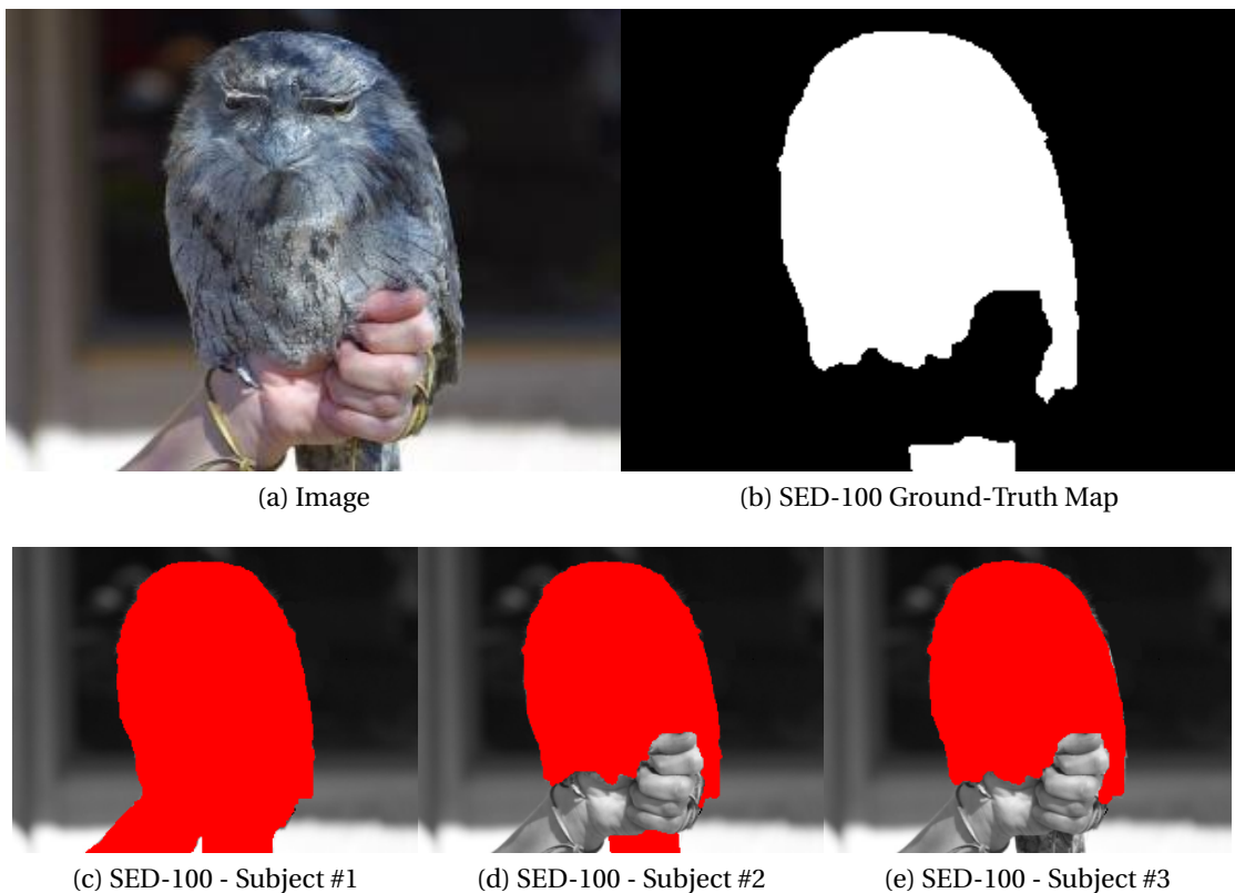
Figure 2.3: (a) Each image in the SED-100 dataset are shown to three subjects. They were asked to (c)-(e) segment the salient object. (cb) The pixels, which are marked by more than one person, are considered as salient in the ground truth map of SED-100 images.
