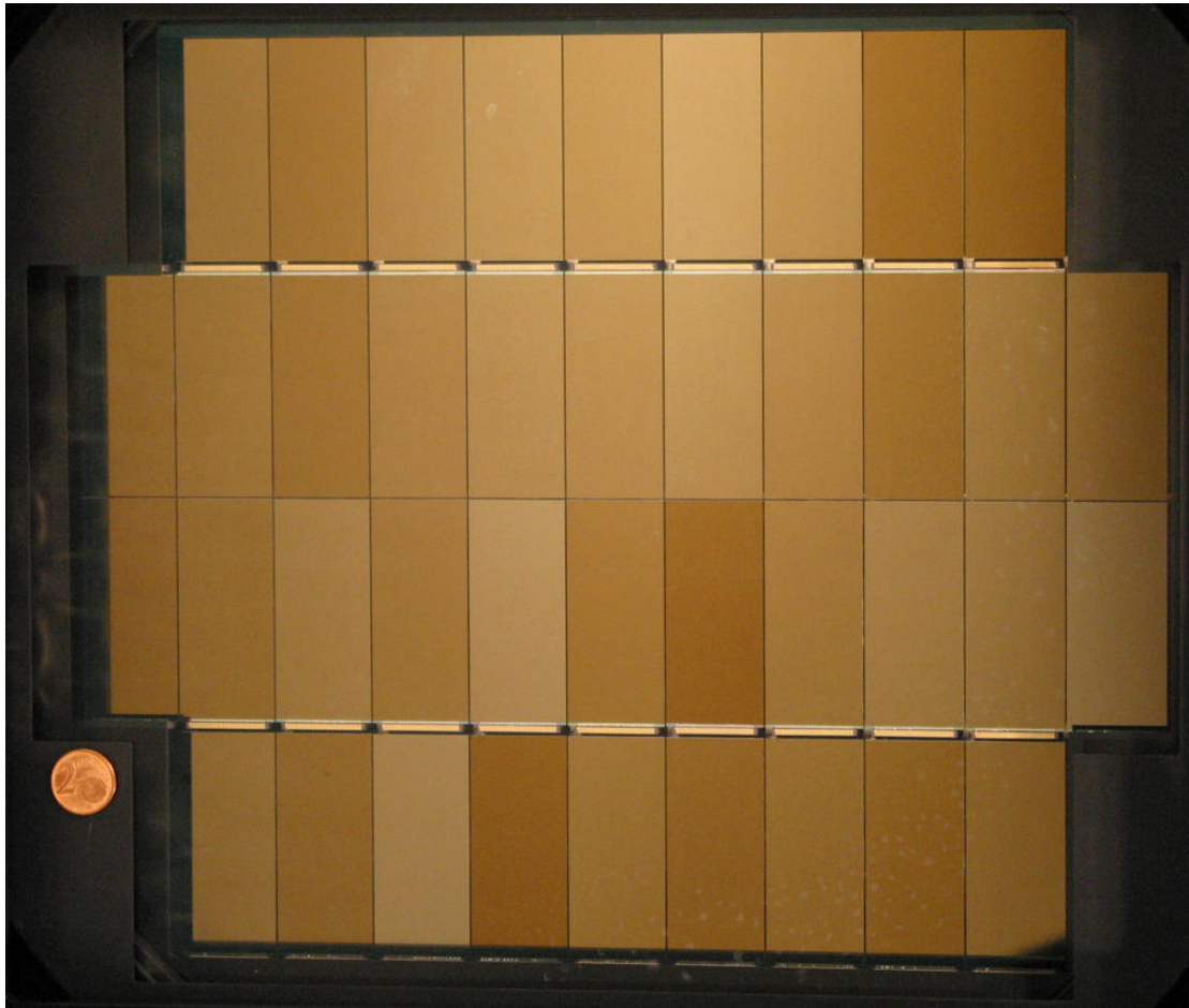
Figure 2.4 – The 40 CCDs mosaics at the heart of MegaCam. The size of the square area is 25x25 cm. The two large gaps between the the 1st and 2nd row of CCDs, and the 3rd and 4th rows are well visible. A 2 cent euro coin is shown for scale.
