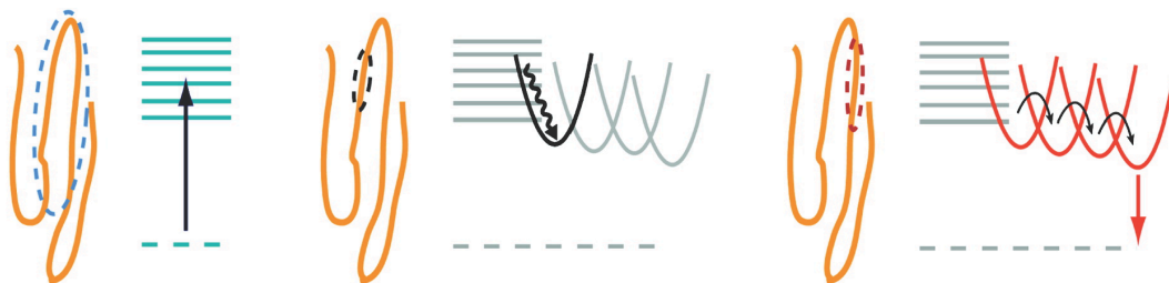
Figure 1.6 Description of the evolution of the polymer excited state in a single chain: initial delocalization, localization of excited states, in the end hops between chromophores. Adapted with permission from (21).
