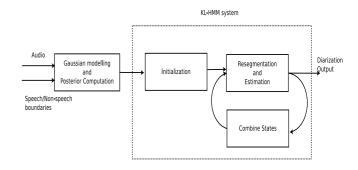
**Fig. 1**. Block diagram representing KL-HMM based diarization system. Multiple iterations of resegmentation and estimation are performed before merging two states
