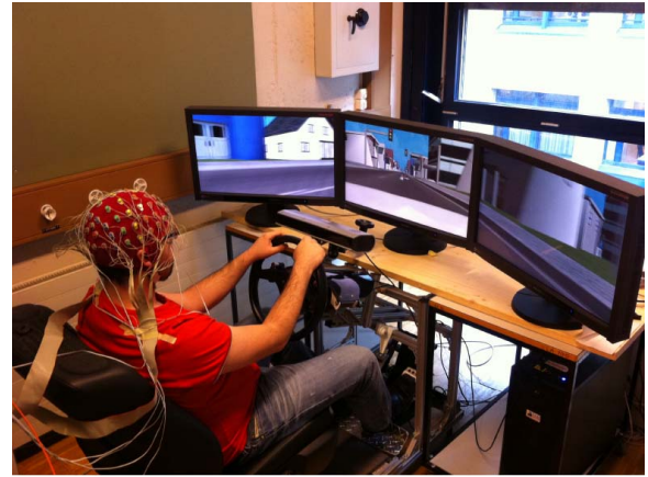
Fig. 2. Experimental protocol. Realistic car simulator including steering wheel, car pedals and three 3D monitors showing the virtual road environment. The subject wearing a 64-channel EEG cap can also be observed.
