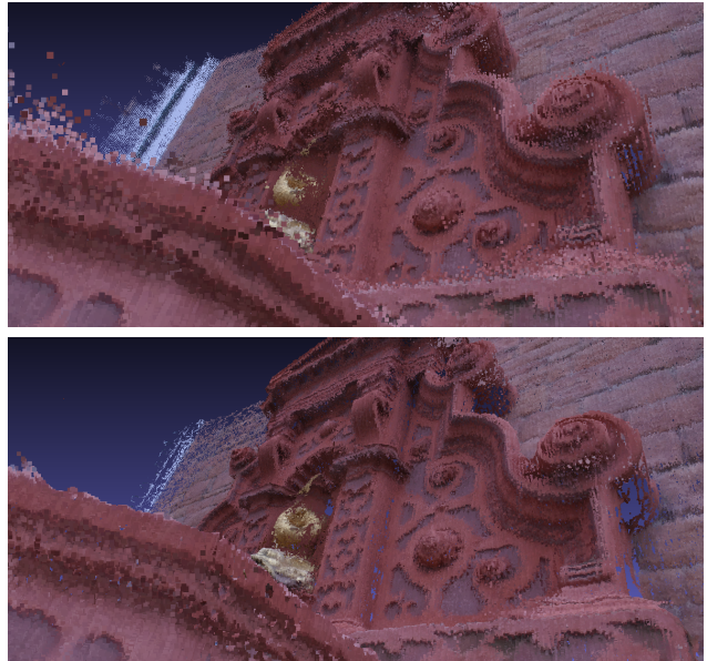
Figure 1. Result of the proposed denoising process on a real-world example. Top: a noisy point cloud obtained using a state-of-the-art Multi-View Stereo reconstruction technique. Bottom: the point cloud obtained after processing with the proposed graph-based denoising methods.
