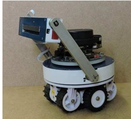
Figure 2. The MarXbot consists of the gripper, LIDAR, computer board, base modules.
