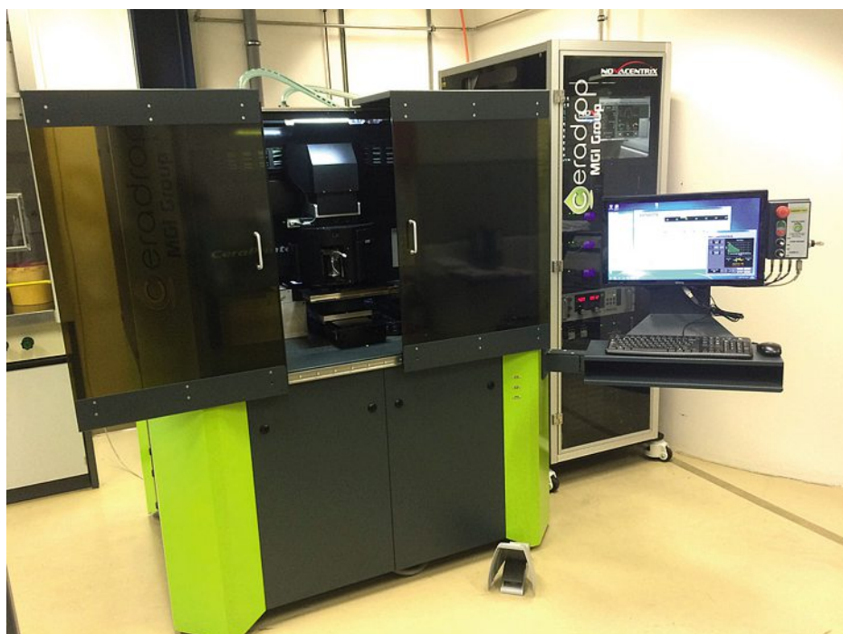
Fig. 6. In the new EPFL campus 'Energypolis' in Sion, LEPA employs an X-Series inkjet printer from Ceradrop with three printheads and an integrated PulseForge 1300 photonic curing station.
