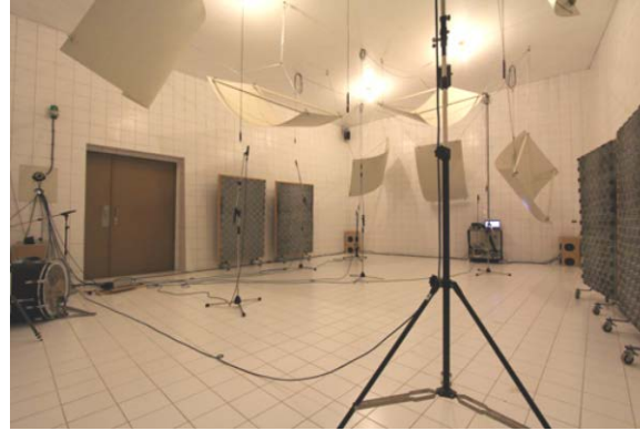
Fig. 4 – left: 2D representation of the reverberation chamber and measurement points; right: picture of the setup (2 electroacoustic absorbers can be seen on the two opposite corners, namely corner C and D)
