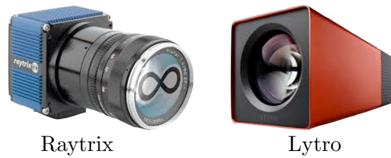
Figure 3.7: Commercial light field cameras. Left: Raytrix camera achieves higher spatial resolution by using three layers of microlenses. Right: Lytro sacrifices the spatial resolution to increase the angular resolution.
