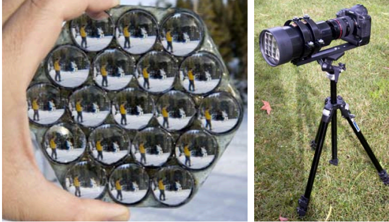
Figure 3.10: Light field camera using an array of prisms and negative lenses [54]. The prisms have different deviation angle to project an array of virtual images corresponding to different angular views on the sensor.
