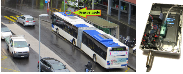
Fig. 2. One sensor node anchored on top of a public bus (left). One of the LDSA sensing modules (right).
