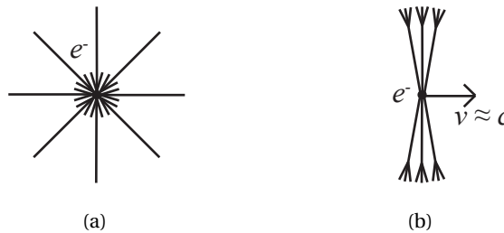
Figure 2.1 – The electric field line force in vacuum in the laboratory frame of (a) a free particle at rest, and (b) a relativistic electron.
