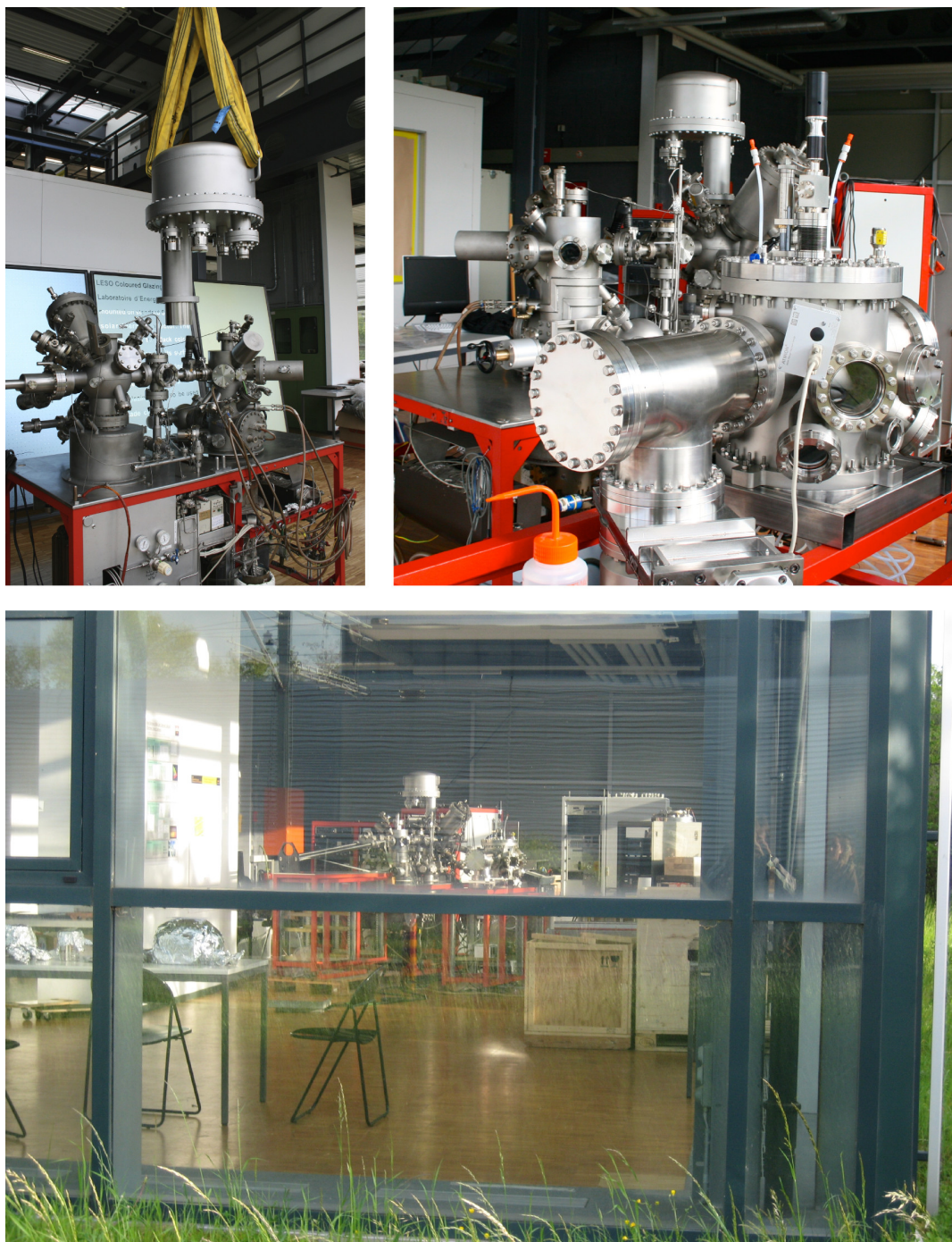
ESCA refurbishment at LESO-PB, re-installing the aligned energy analyser, and first reference spectrum before christmas (May to December 2010).
