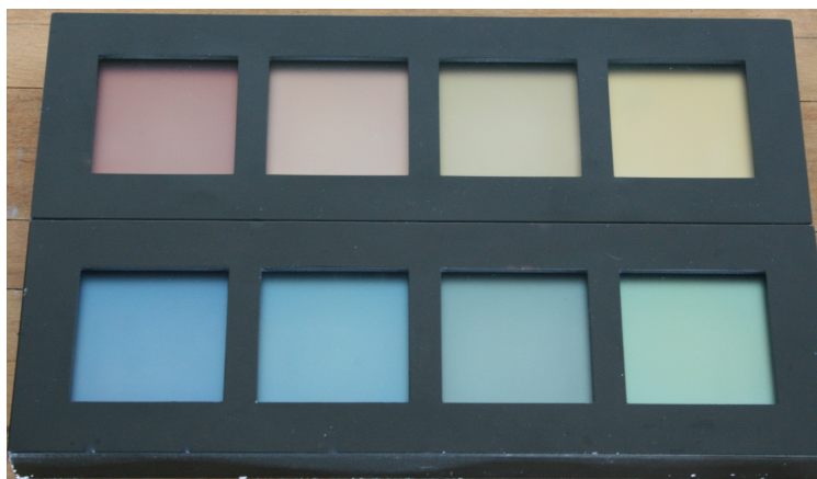
Figure 4.10: Homogenous coloured samples 6 \times 6 \text{ cm}^2 with sputtered multilayer coatings on the reverse side of the glass. Front side is chemically etched for light defusing.
