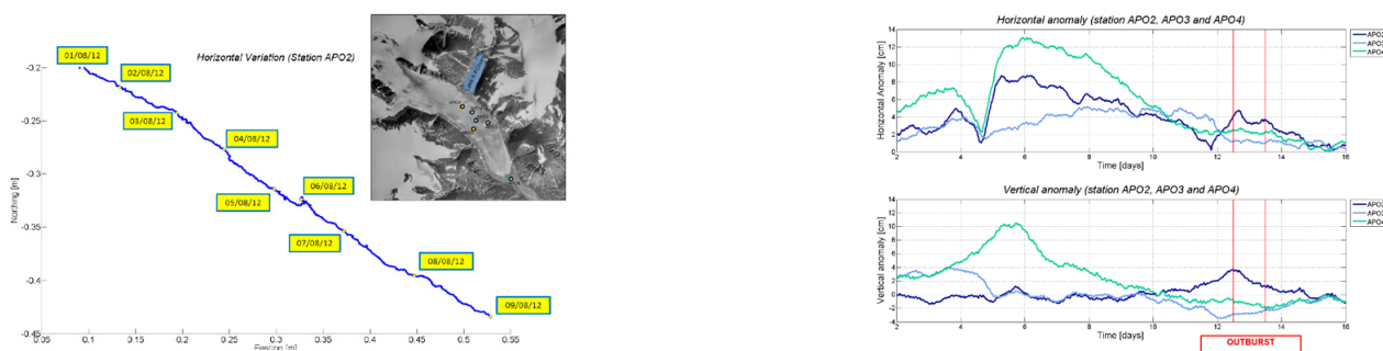
Figure 1 Horizontal displacement during the GLOF-period in 2012 (left). Horizontal and vertical motion anomalies of stations 2, 3 and 4 during initiation phase and outburst of the GLOF.
