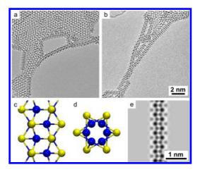
Figure 6. 2D to 1D transition resulting from prolonged electron irradiation. (a and b) AC-HRTEM images of MoSe nanowires suspended over holes in the 2D MoSe₂ layer. (c and d) Side and end projection of a DFT relaxed structural model of the nanowire. (e) Simulated HRTEM image of the nanowire.
