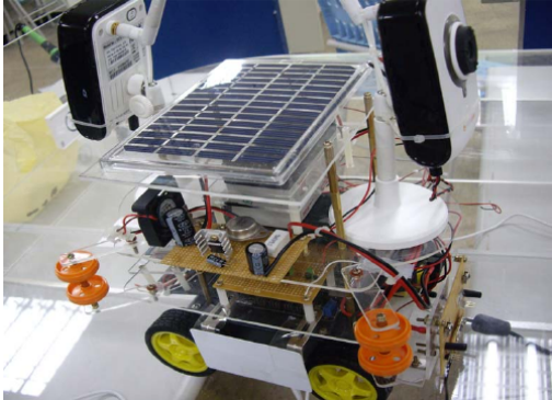
(d) Indoor surveillance security robot using a solar panel. Picture credits: H.T. Lee, et al. [124].
