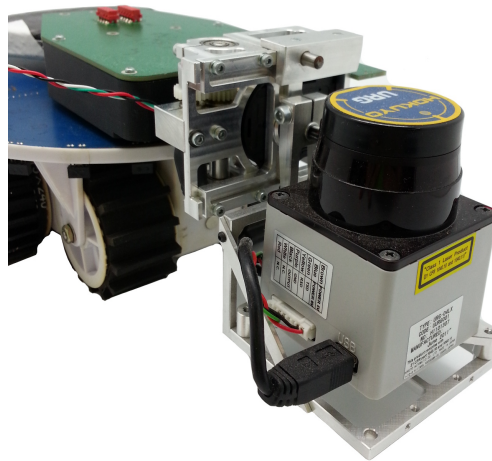
(b) Picture of the Hokuyo module, mounted on top of the mobile base.
