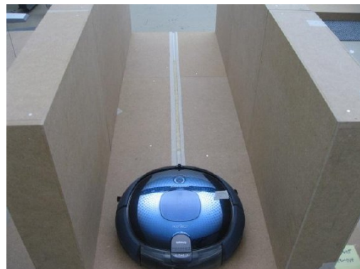
(f) Robot 4 during the crack cleaning test.
