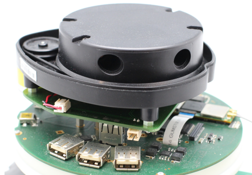
(b) Picture of the Neato module, mounted on top of the processor board.
