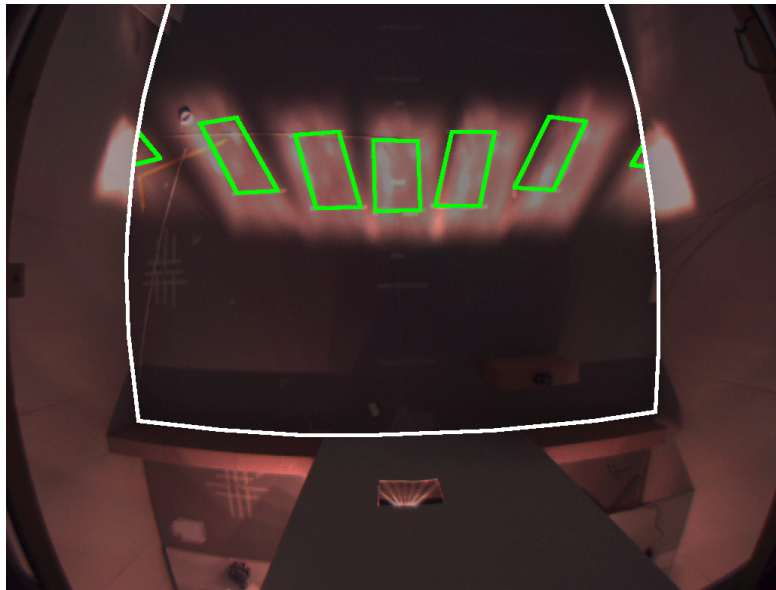
(a) Fused images as seen from the overhead camera when the light source moves from one hour to the next. Green rectangles: Position given by the software simulation. White line: Room's boundaries.
