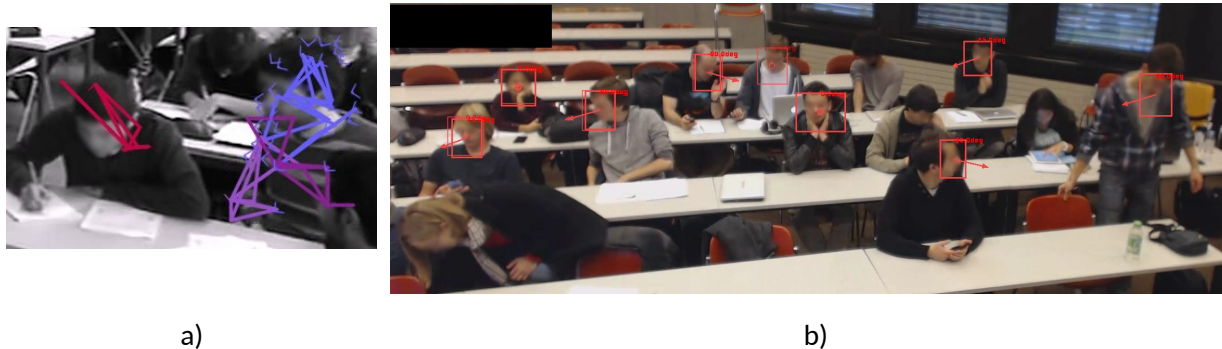
Figure 1: a) Motion vectors visualized on top of the students. Individual vectors are grouped into motion paths depicted as lines of different colors. b) Head detections and estimated gaze directions for a group of students in the classroom.
