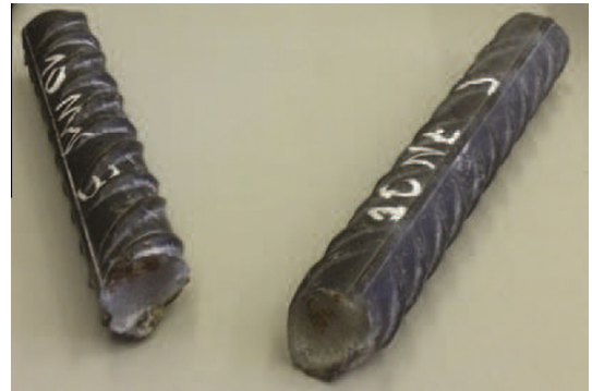
Fig. 13. Failed rebars due to fatigue.
