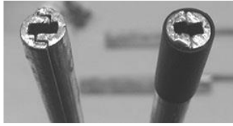
Fig. 2. The copper profiles of the ‘S’ (left) and ‘Plus’ (right) strands.
