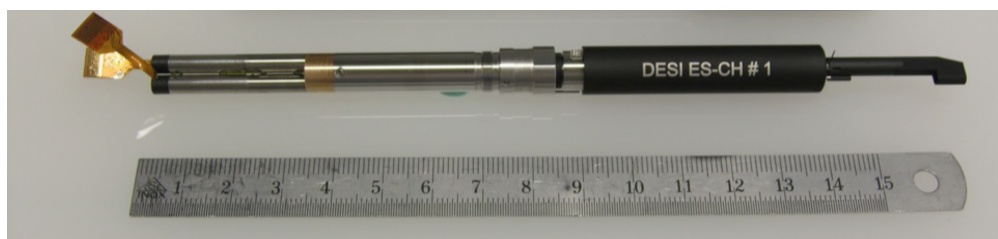
Figure 1.2: A fiber positioner robot developed in collaboration between EPFL and UAM [11; 12].
