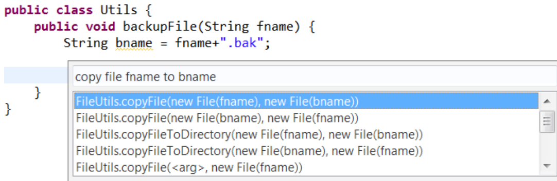
Figure 3.1: After the user inserts text input, anyCode suggests five highest-ranked well-typed expressions that it synthesized for this input.
