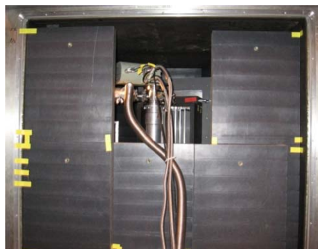
Figure 16: The final shielding of the detector tank, (before closing the doors of the analyzer housing as much as possible) leaving only a necessary hole for the CTI tubes and wires.
