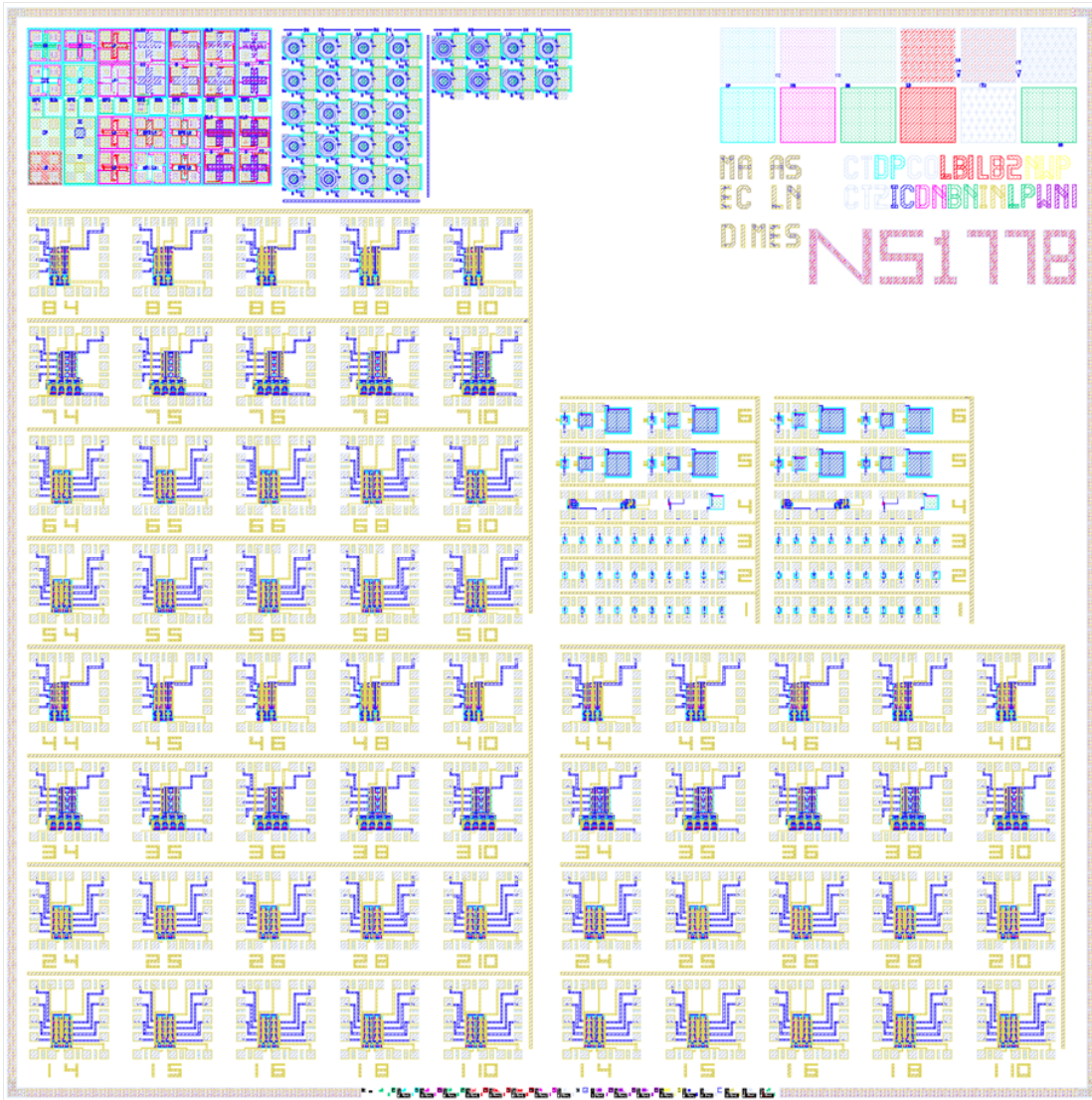
Figure 4.5: Full chip layout of different 4 \times 4 Ge SPAD arrays.
