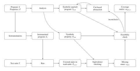
Fig. 2 Flow diagram of PBCOV
