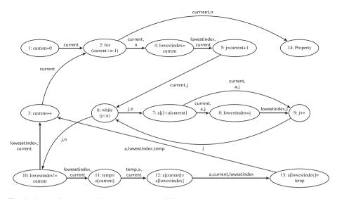
Fig. 6 Control flow graph of the sort example of Fig. 1
