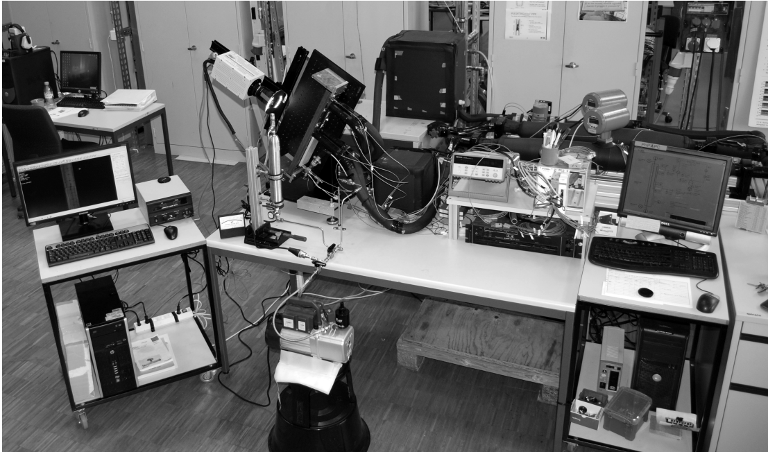
Figure 3.1: CLPHP experimental facility
