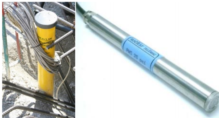
Figure 7:5 Reading head of a borehole extensometer embedded within the raft (left) and the PWS piezometer from ROCTEST™ (right)
