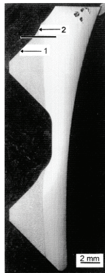
Figure 2-4 Gripper latch arm showing the two areas where wear occurs 1) straight 2) transition zone in curved shape [9].
