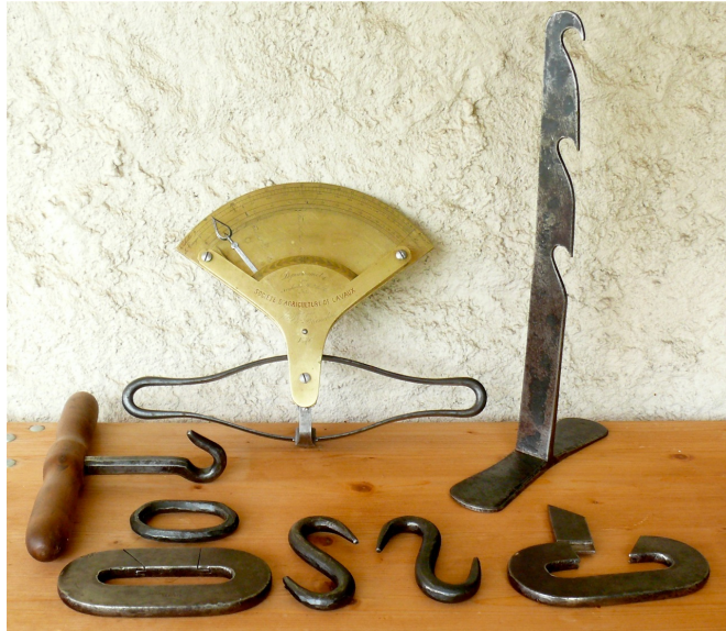
Dynamometer with accessories, by Arnheiter, the mechanic who had worked for Regnier. Private collection of J.-F. Loude
