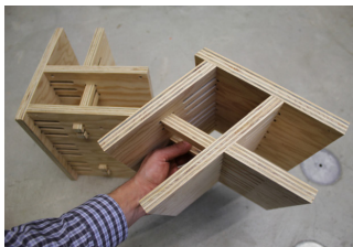
8 Prototype for a Snap-fit Jointed, Double-layered Corner ( 90^\circ and 120^\circ fold)—built from 17mm plywood, 75mm spacing. Note the double-snap-fit element, which has a hook for the first layer and another hook for the second layer. The snap-fit joint in the middle is used as a spacer element. This technique can be used for structural improvement as well as for the fitting of (flocked) insulation materials
