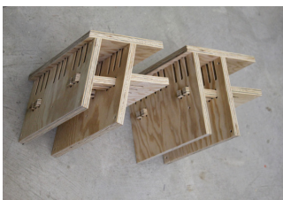
7 Sandwich Element with Inclined Vertical Connectors—The snap-fit joint allows for a simple, precise and quick assembly of non-orthogonal connections. There is no difference between the fabrication and assembly of a 90^\circ joint and a 110^\circ joint. This can be exploited for the assembly of corrugated sandwich components
