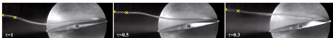
Fig. 6 Superposition of the cavitating TLV visualizations during 11 ms for three gap widths. The yellow crosses represent the position measured by SPIV in cavitation-free regime, in the planes z/c = 1 and 1.2 . Flow conditions: W_\infty = 10 m/s, incidence = 10^\circ , p_\infty = 1 bar
