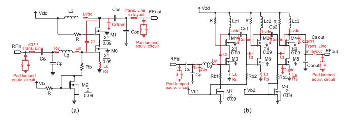
Figure 6. Parasitic schematic of the single-stage and three-stage LNAs. (a) 1-stage LNA parasitic schematic. (b) 3-stage LNA parasitic schematic.
