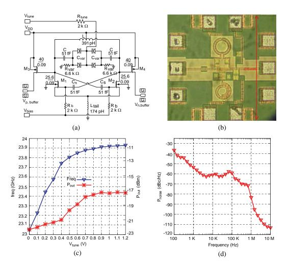
Figure 10. VCO schematic, die photo and measured results. (a) Cross-coupled VCO schematic. (b) Die photo of VCO. (c) VCO tuning range and output power without losses of cables and connectors. (d) Locked phase noise of the designed VCO with commercial PLL chip.
