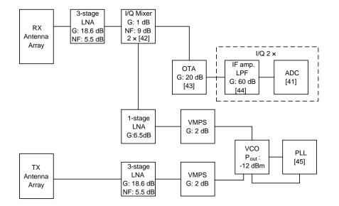
Figure 12. Block diagram in transceiver mode.
