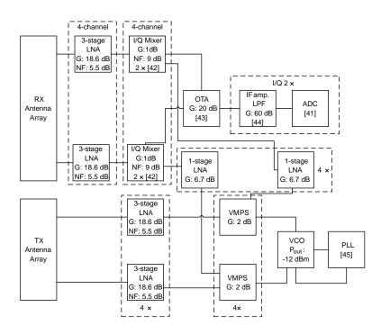
Figure 11. Block diagram in Doppler radar sensor mode.
