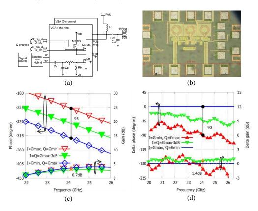
**Figure 9.** VMPS schematic, die photo, simulated and measurement results. (a) Schematic of the VMPS. (b) Die photo of VMPS. (c) VMPS simulated results. (d) VMPS measurement results.
