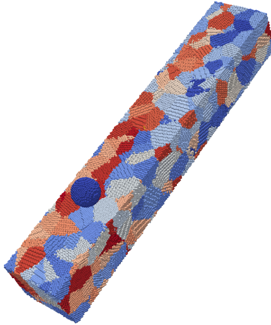
Figure 3.2 – Example of a polycrystalline microstructure. Atoms are coloured by grains which are defined by the cells of a Voronoi tessellation of 200 randomly distributed points in the substrate geometry. Each Voronoi cell is assigned a random lattice orientation and filled with atoms. The structure is heated, annealed under isostatic pressure, and quenched before the indenter is added.
