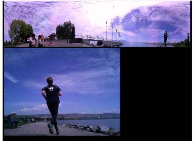
Fig. 11. Omnidirectional snapshot of resolution 1024 \times 256 for the nearest neighbor interpolation technique plus VGA ( 640 \times 480 ) display of a single selected camera.
