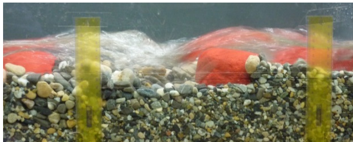
Figure 3.12: Example of an hydraulic jump.
