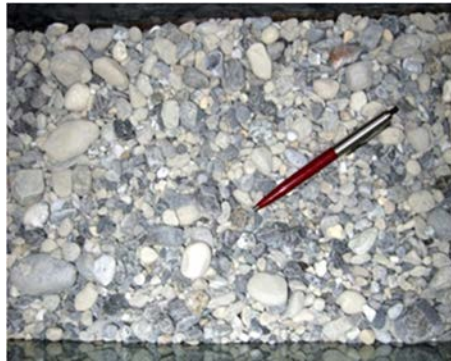
Figure 3.5: Sediments used for the mobile bed substratum.
