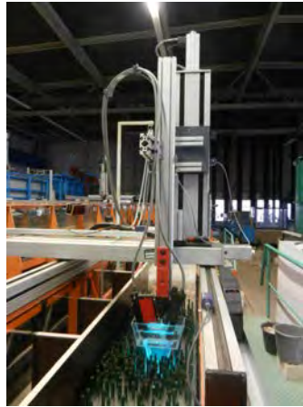
Figure 3.4: Traverse system used at LWI for positioning the LDA probes.
