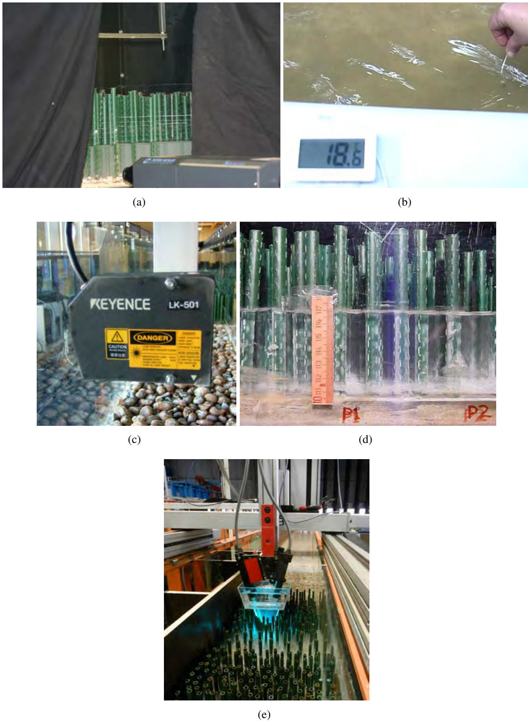
Figure 3.7: a) PIV laser head; b) digital thermometer; c) laser displacement sensor; d) ruler used to measure free-surface levels with video images; e) uEye camera used to measure free-surface levels and f) probes during LDA velocity measurements.
