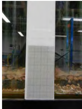
Figure 3.36: PVC sheet used to calculate the calibration factor to convert velocity maps in image units (px/s) into metric units (m/s).
