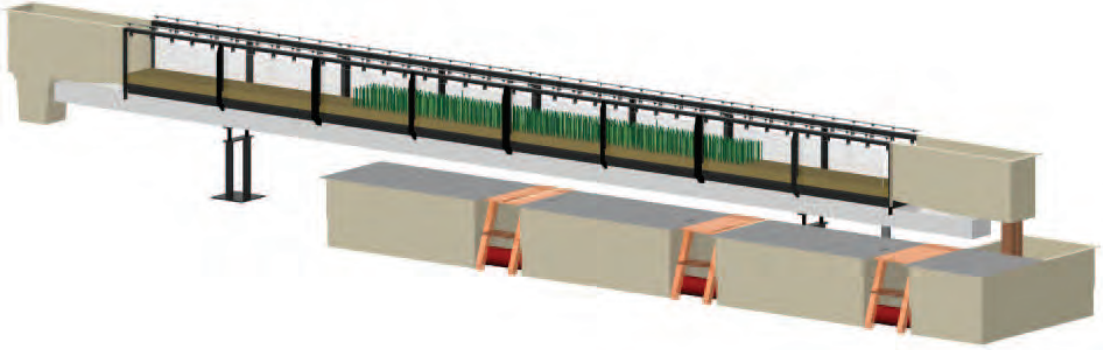
Figure 3.1: Schematic view of the recirculating tilting flume at IST.
