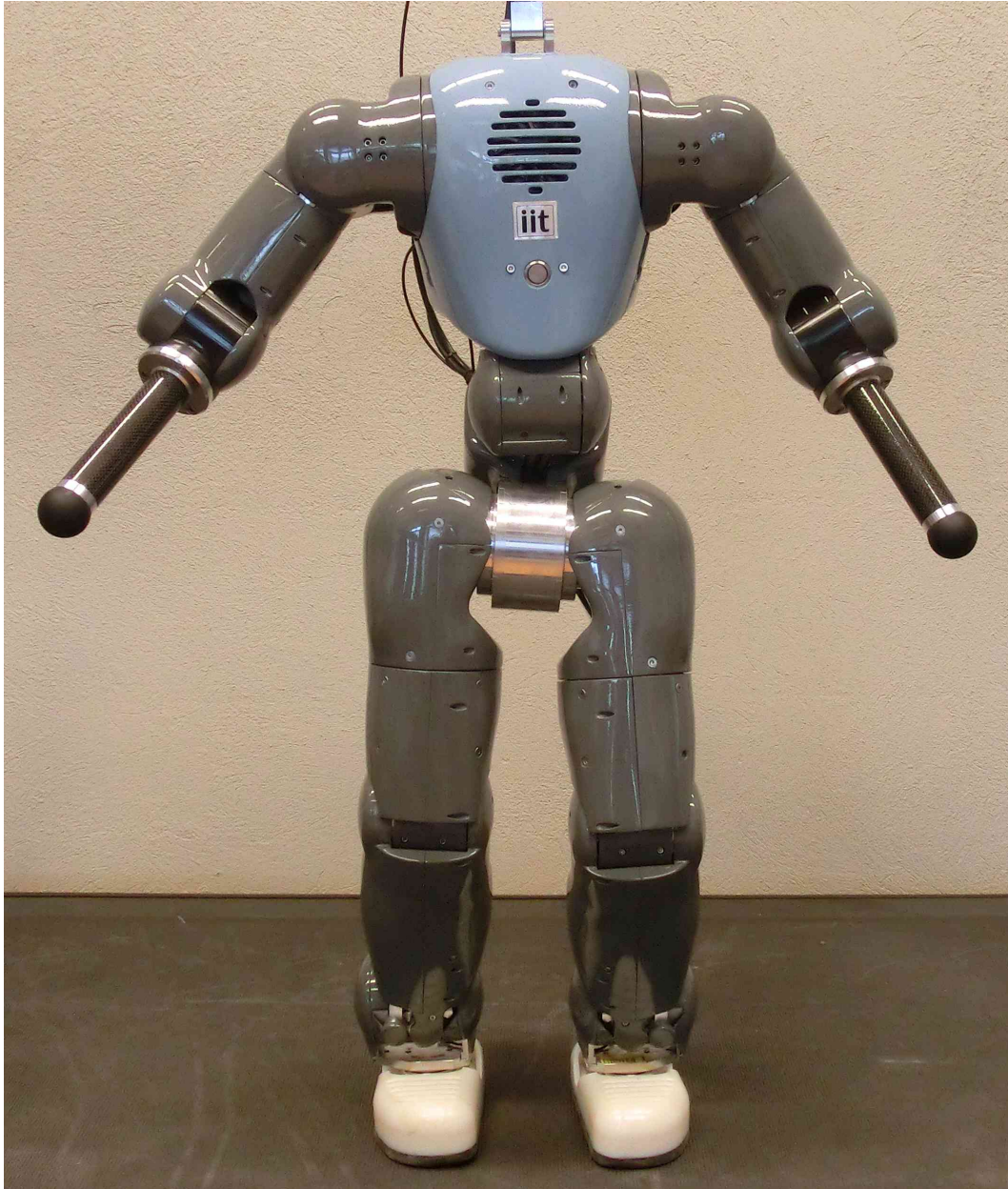
Figure 1: COmpliant HuMANoid Platform – COMAN, developed by IIT, and used in the experiments to demonstrate the possibility of using modified task space control for motion imitation.
