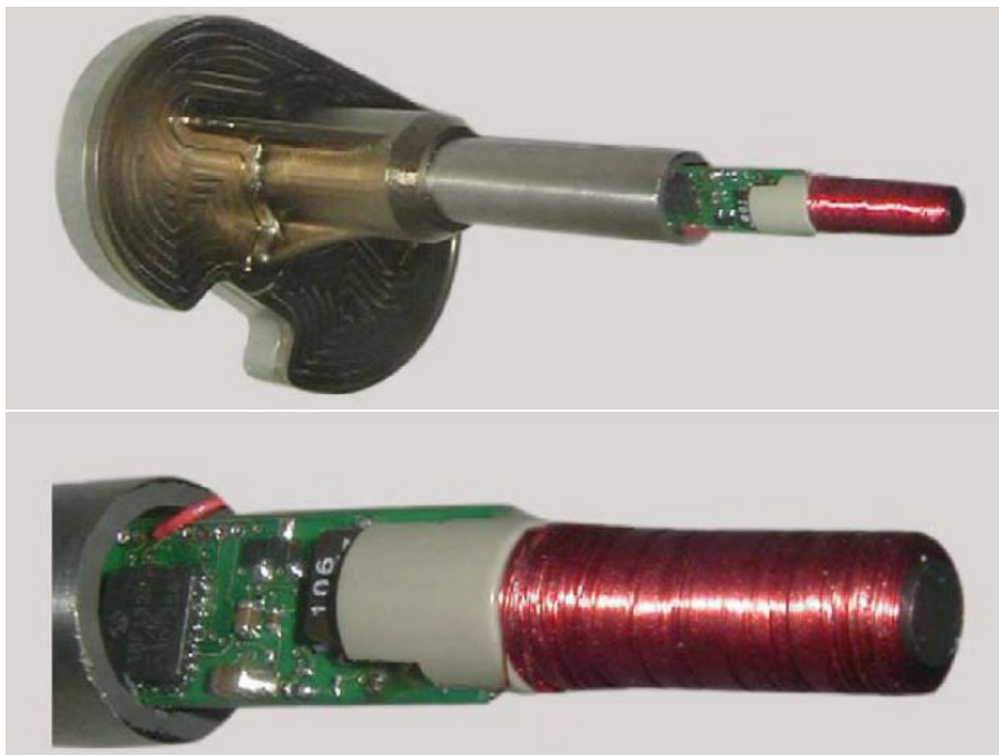
Figure 3.6: (a) Implanted prosthesis with the telemetry system and (b) closed view of the electronics with the antenna. Reprinted from [26].
