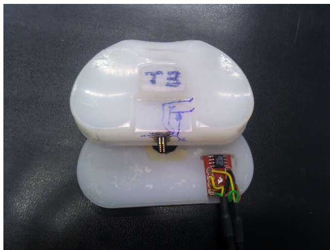
Figure 6.22: PE insert modified to embed the sensors.
