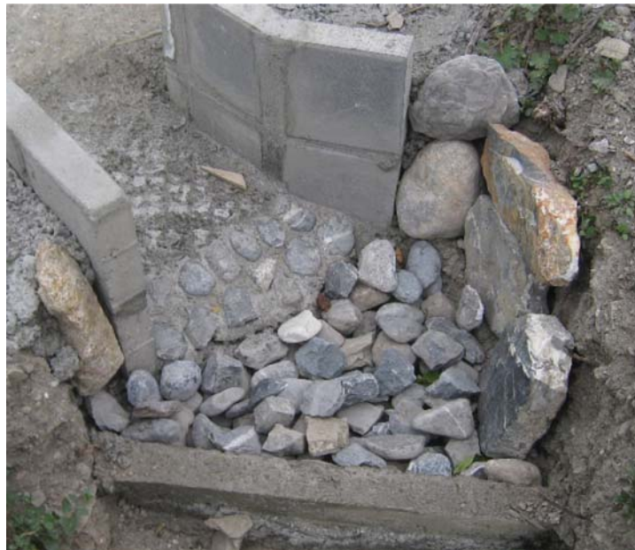
Figure 6. Stilling basin and downstream sill of the physical model.
