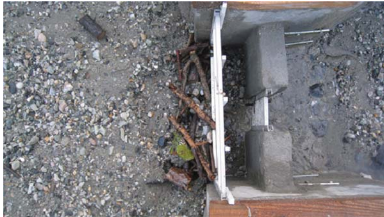
Figure 8. Situation at the dam after 30-year-flood event (physical model, flow from left to right).
