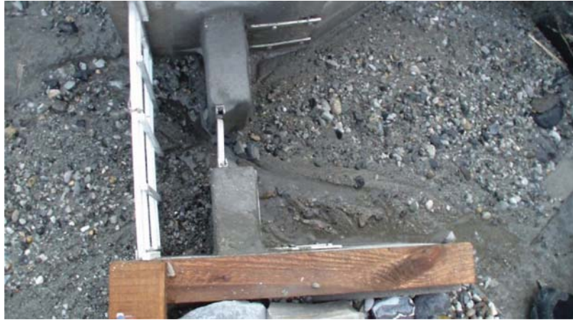
Figure 7. Situation at the dam after 10-year-flood event (physical model, flow from left to right).
