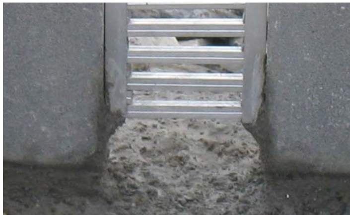
Figure 4. Bottom opening and upper flow section with horizontal beams on the physical model.
