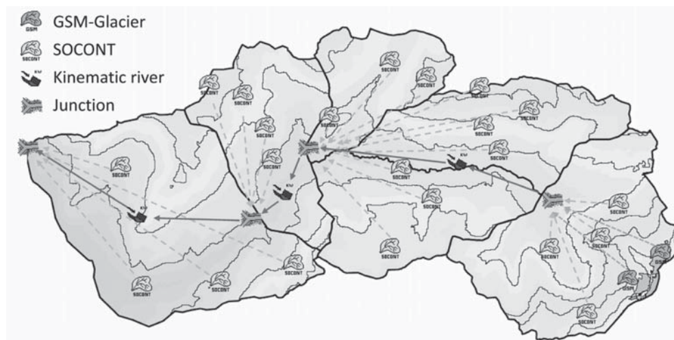
Figure 2. Sub-basins and elevation bands in the Grande Eau watershed (tributary in the downstream part of the Upper Rhone River basin) and their schematic representation as glacier and non-glacier bands, rivers and junctions.
