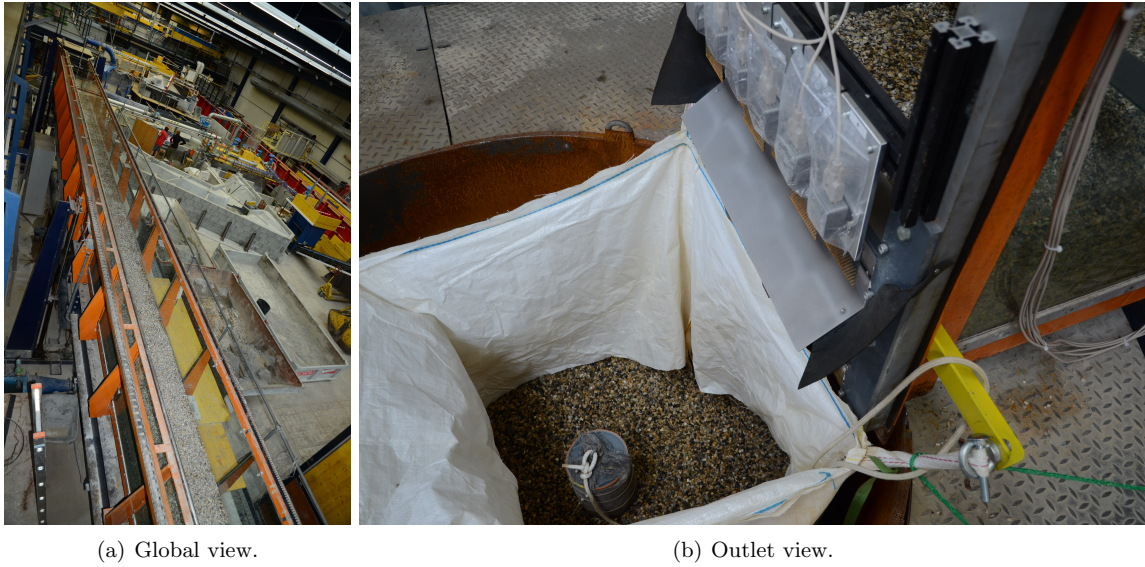
Figure 3.12: Armfield flume. (b) Note the six accelerometers for the recording of bedload transport rates at the top of the image and the construction bag to retrieve and weigh the accumulated sediments.
