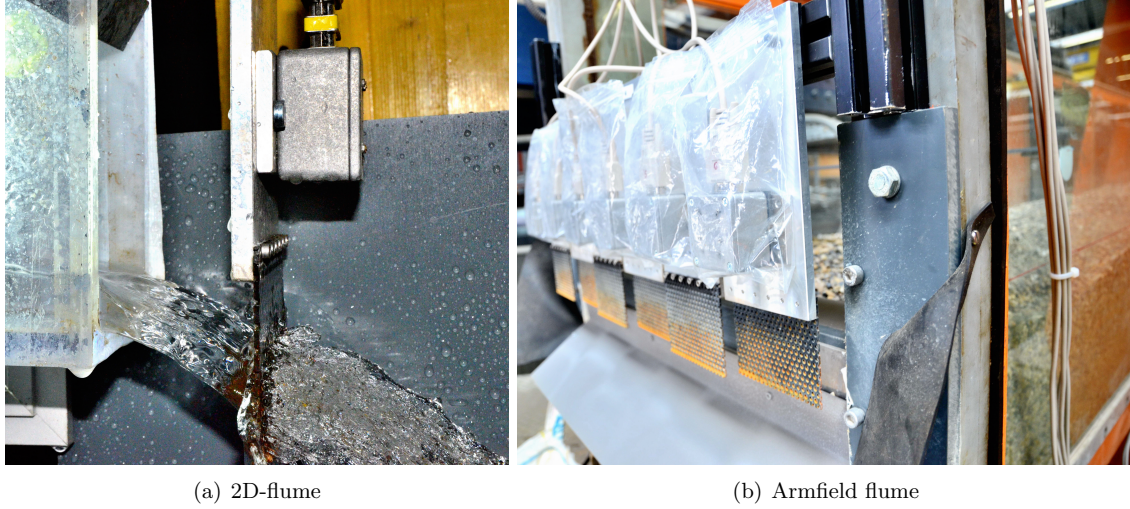
Figure 3.2: (a) Picture of an accelerometer measurement system placed at the outlet of the 2D-flume (with water flowing from left) used for bedload measurements. The accelerometer recording the particle impacts is fixed on the backward face of the plate and is protected by a metallic box. (b) The 6 accelerometer measurement systems placed along the width of the Armfield flume outlet (without water flow, downstream direction is from right to left).
