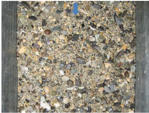
Figure 7. Tributary bed substrate in equilibrium for the reference configuration.
