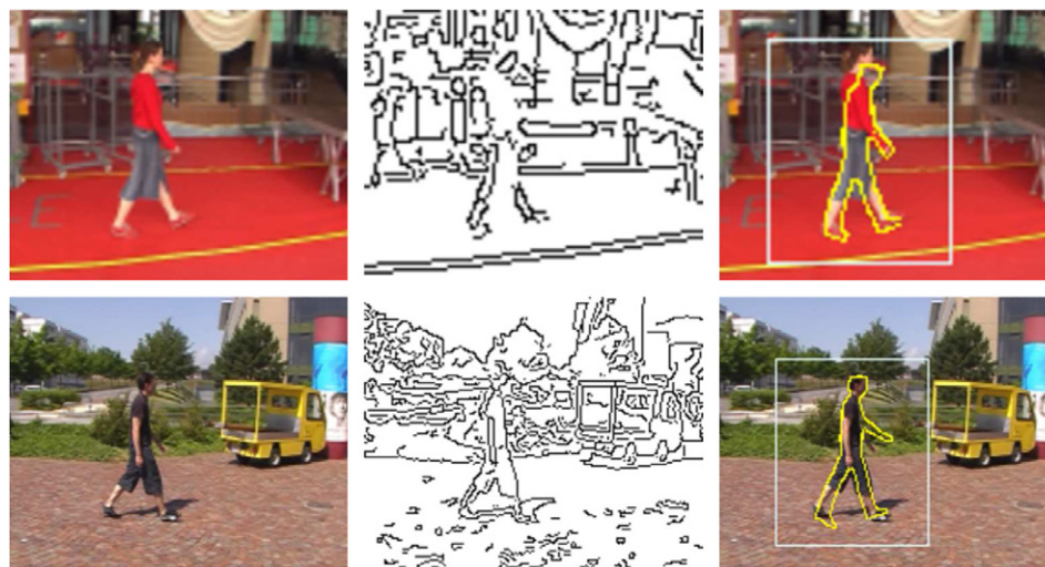
Fig. 11. Robustness to changes in clothing. First row: the subject is detected even though she wears a shirt. Second row: correctly detected person wearing knee-length pants.
