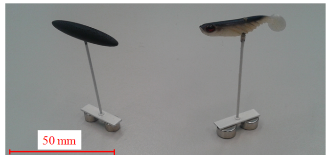
Fig. 6: Lure modules. Left: a rigid black ellipsoid lure. Right: a soft fishing lure. The base is painted in white so it is merged with the white background inside the aquarium.
